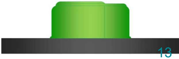
The complete bolt has to be covered with Wrappingband.
