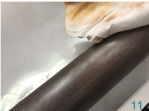
Surface cleaned with SFL® Cleaning Wipe.
