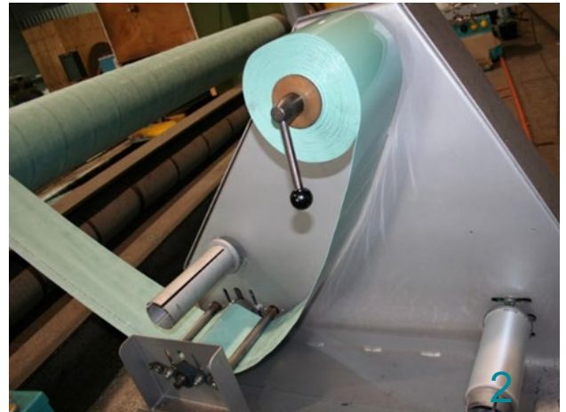
Depending on pipeline diameter, the angle of the FAST Basecoat Wrapping Device must be adjusted to ensure a minimum 10mm side-by-side overlap.
