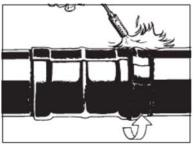
Shrink the leading edge sleeve down by moving the torch all the way around the pipe in a paintbrush motion. Make sure the sleeve has fully shrunk and adhesive flow is evident on both edges.
