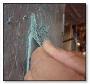
At least one EasyQote®SC Reference Patch Test must be made prior to EasyQote®SC Patch application on site. Site QC or STOPAQ Trained Inspector can determine any other reference patch amount above the minimum requirement of one reference patch recommendation from ACT.
