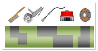
2.5.3. Perform Surface Cleanliness/Reference Patch Test to confirm the surface has been cleaned to a minimum St2/St3 standard, and ready for EasyQote®SC Patch Application.
