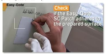
3. Cohesive failure should occur and the remaining EasyQote®SC Reference Patch material should cover ≥95% of the surfaces. If this is less, further cleaning is required. Repeat cleaning and cleanliness check until ≥95% of the surface remains covered with residual EasyQote®SC Reference Patch product.
