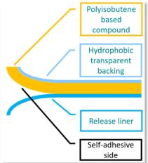
Remove the release liner (in this instance the product will be removed from the siliconised cardboard) just prior to application to the surface to avoid contamination of the adhesive surface and premature adhesion to the substrate.
