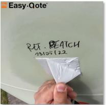
Below are examples of peel test failures (adhesive failure) as seen from prior STOPAQ Application which is applicable to the EasyQote®SC Reference Patch application process:
