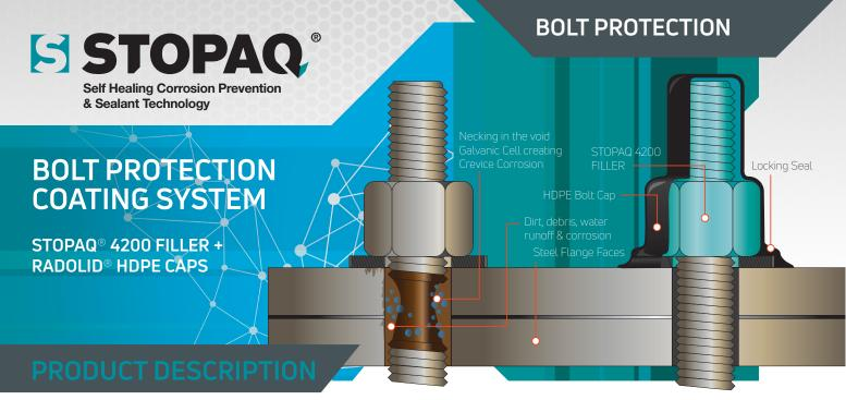
STOPAQ® 4200 Filler is a non-toxic, highly viscous, surface tolerant, single component, non-reactive injection filler with corrosion preventing properties designed for filling and protecting hard-to-clean corrosion sensitive areas where water can accumulate. It has a wide service temperature range, excellent
